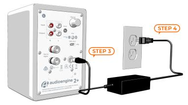
4. Connect the AC power cord to the other end of the power supply and plug the cord into a functioning power outlet. A light on the power supply should be illuminated.
