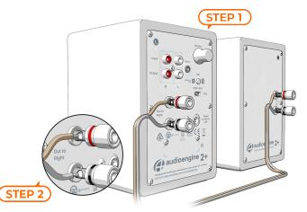
2. Connect the included speaker wire to the A2+ left (powered) speaker terminal and to the right (passive) speaker terminal.
