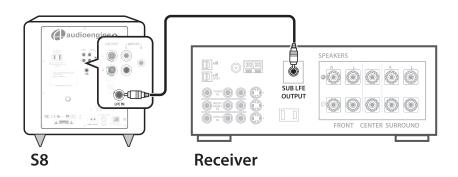
Note: Your receiver's manual should indicate which subwoofer connection is most appropriate.
