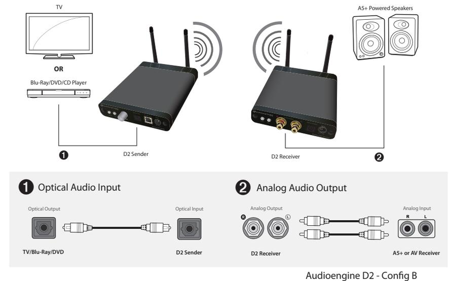
Step 1 -- Connect an optical output of your computer, TV, Blu-Ray, DVD, etc. to the optical input of the D2 Sender.
